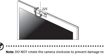
**Note:** DO NOT rotate the camera clockwise to prevent damage to the device.
